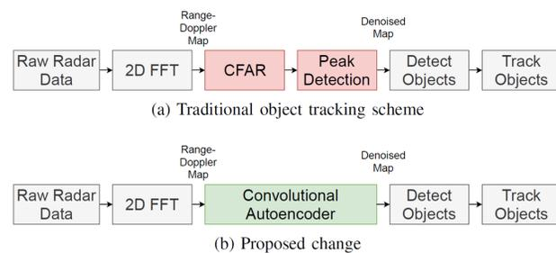
Figure 1: Simplified schematics of the traditional tracking and the proposed change.
