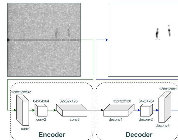
Figure 2: Noisy Range-Doppler map passing through a 3 layer encoder and 3 layer decoder to obtain a cleaner image.
